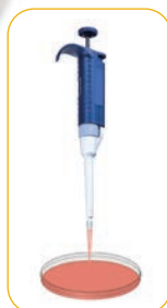
Aspirate sample into 1000µl tip
