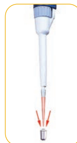
Press FLOWMI onto pipette tip
