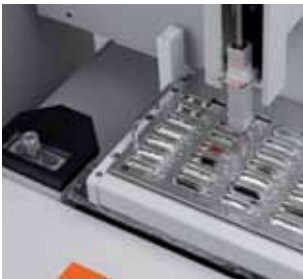
▲ A multi-matrix autosampler for vertical and horizontal applications saves working time ▼
